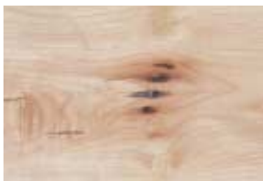
BIRD PECKS: Small blemishes in the grain pattern resulting from birds pecking that sometimes contain ingrown bark. An exception to the rule is hickory and elm.
