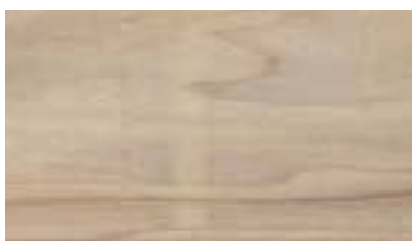
STICKER MARK: The mark left on the board from a seasoning sticker, which can be removed in the surfacing planing process.
