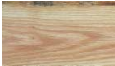
HEARTWOOD and SAPWOOD: Heartwood is the mature wood, which is often darker, extending from the sapwood to the pith. Sapwood is the lighter coloured wood growing from inside the bark to the heartwood.
