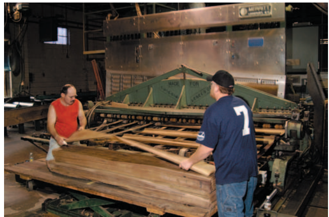
Figure 1.—A veneer slicing operation showing the flitch or half log (upper right) being moved downward against a knife. The resulting veneer is being conveyed forward and stacked in order.
