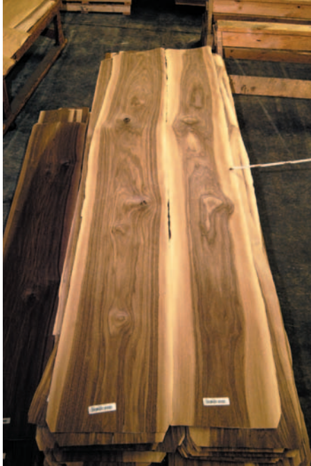
Figure 4.— Two sample sheets from a walnut flitch showing numerous problems. Knots and irregular grain patterns are present throughout. The color is not uniform and the sapwood is excessive.
