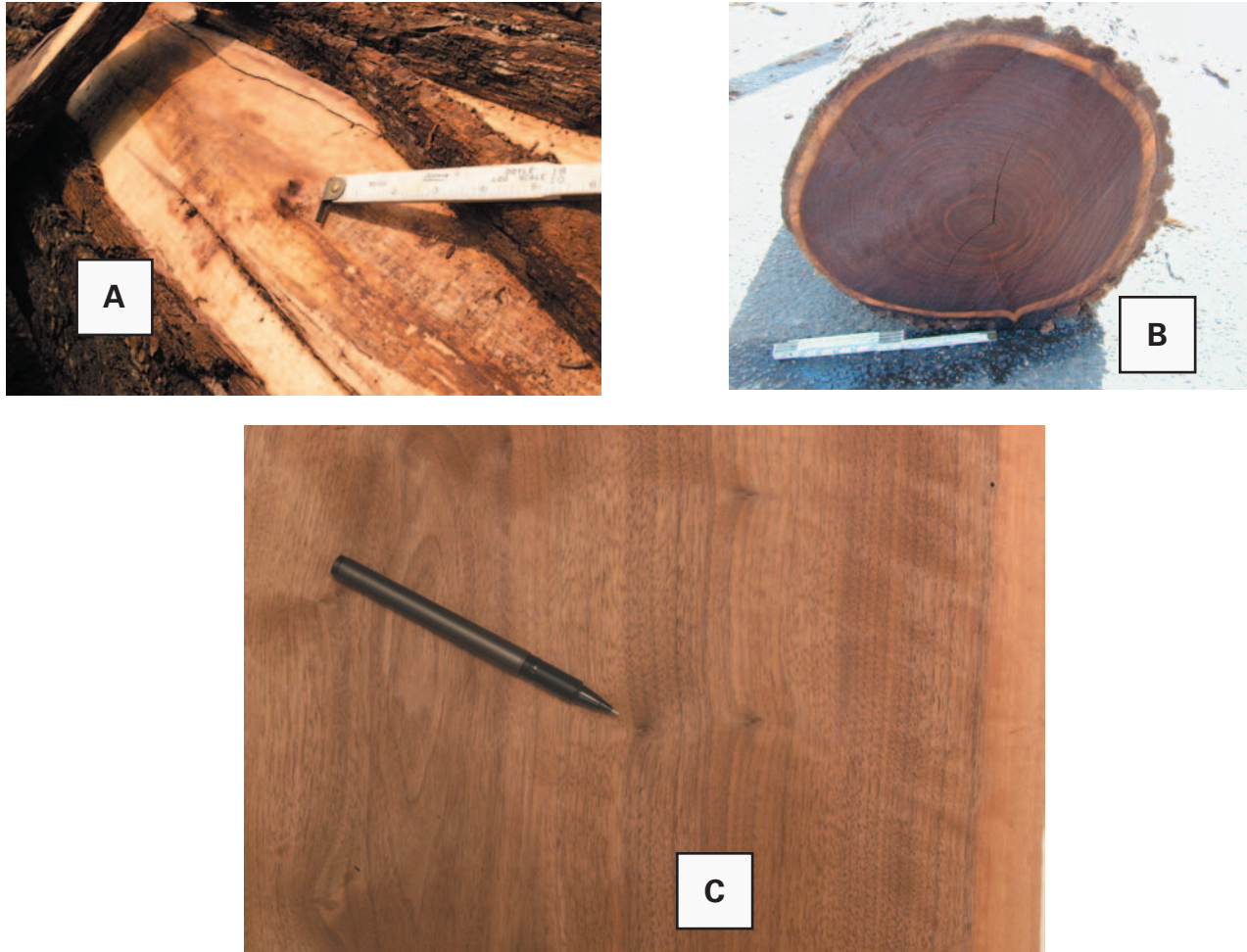
Figure 6.—Pin knots in walnut. (A) shows an easily seen pin knot on a debarked surface of a log. These pin knots are hard or impossible to detect unless the bark is removed or the log is cut (B) from the tree. They will appear as a spot on flat sliced veneer (C) and as light streaks on a quartered surface (B).
