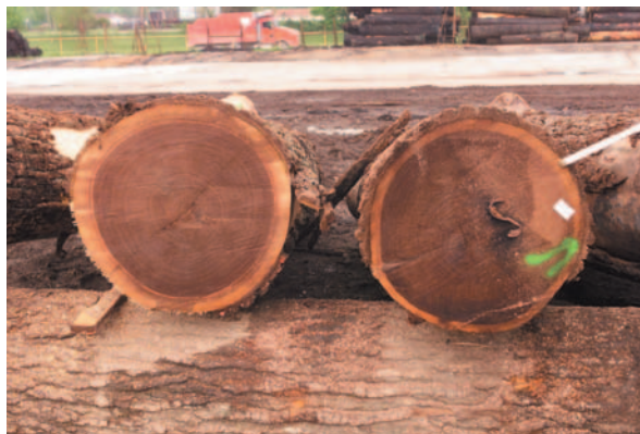
Figure 7.—Wide (left) and narrow sapwood on two walnut logs. Sapwood is considered a defect in walnut veneer.
