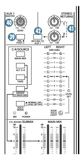
So, the original "dry" signals go from the channels to the main mix and the affected "wet" signals go from the STEREO RETURN to the main mix, and once mixed together, the dry and wet signals combine to create a glorious sound. So, armed with this knowledge, let's visit the Auxiliary World:
