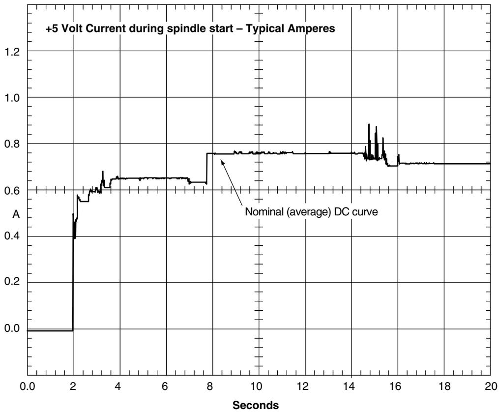
Figure 6. Typical ST39204 drive +5 V current profile
