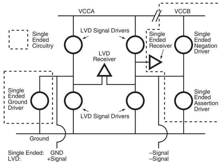
Figure 25. Typical SE-LVD alternative transmitter receiver circuits
