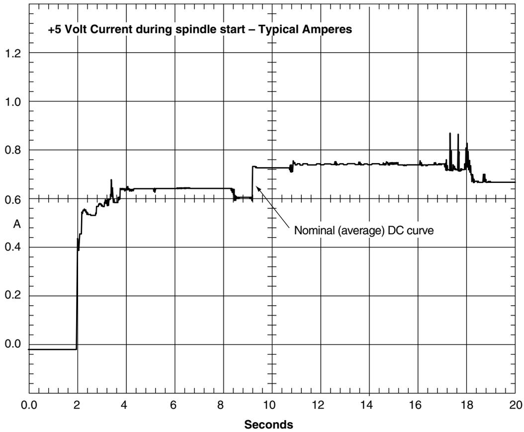
Figure 5. Typical ST318404 drive +5 V current profile
